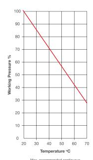
Max. recommended continuous working temperature = 60°C
