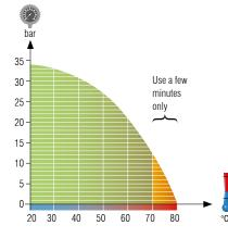
MAXIMUM WORKING PRESSURE 20 BAR AT 70°C
